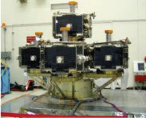
Figure 7: Probes on Probe Carrier at JPL
