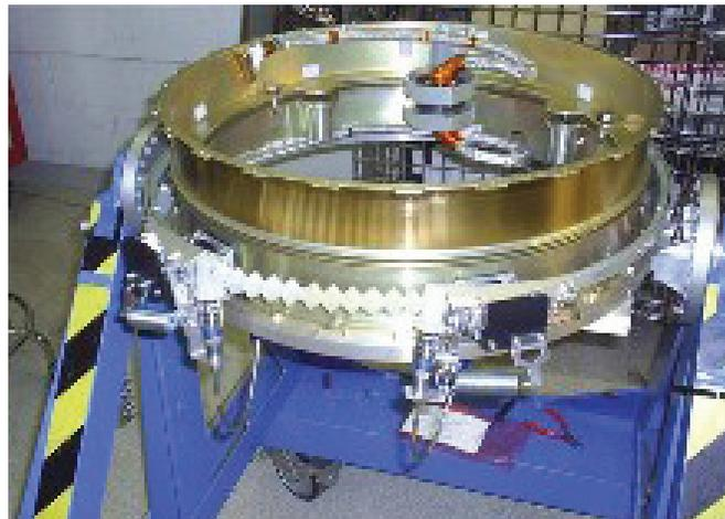
Figure 6: Separation System in Test
