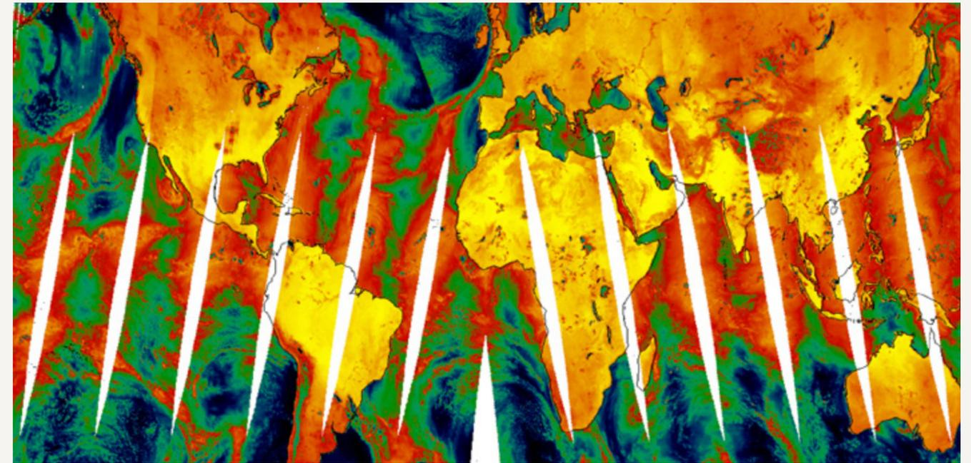
The Microwave Sounder instrument on board Metop-SGA satellites will improve the accuracy of weather forecasting by providing data relevant for observing atmospheric temperature and water vapour in clear and cloudy conditions
