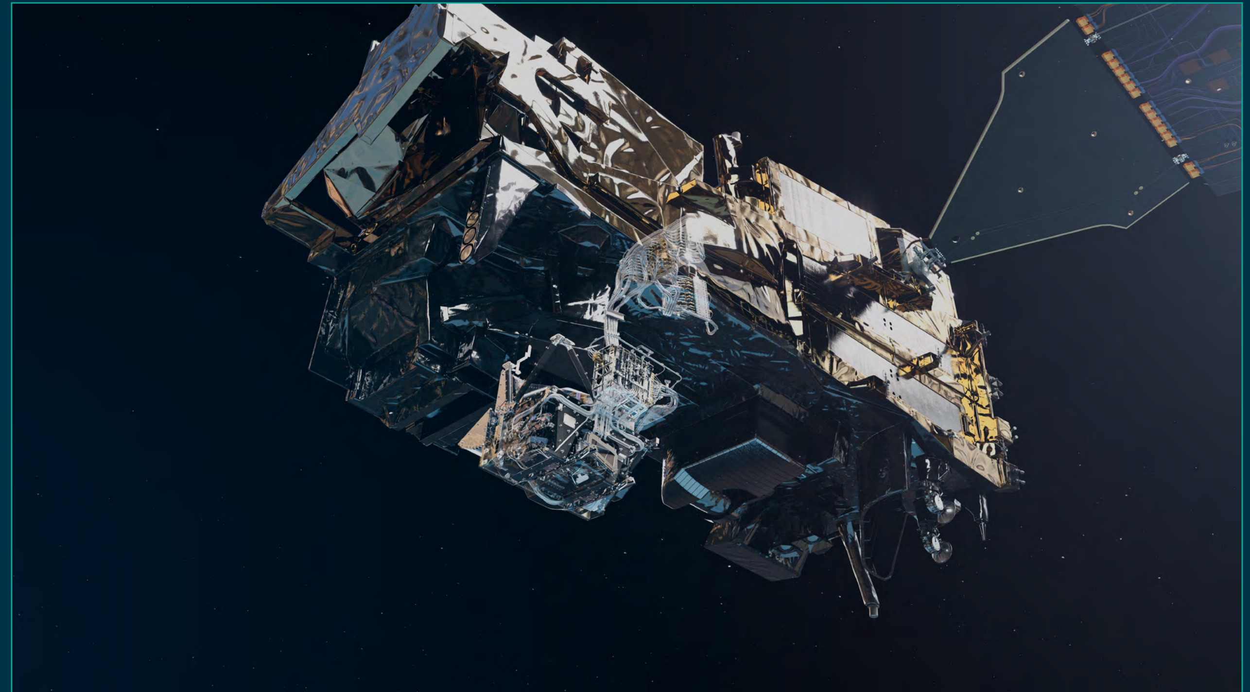
Sentinel-5 will orbit at 832 km in a polar orbit, complementing the geostationary Sentinel-4.
