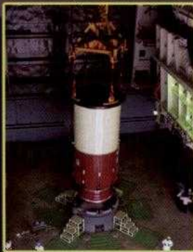
Core Base Shroud + Nozzle end segment stacking at VAB
