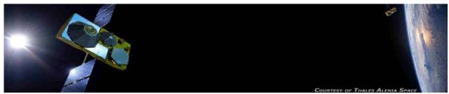
The new Globalstar second-generation low-earth-orbit (LEO) satellite is a three-axis stabilized spacecraft consisting of a trapezoidal main body with two solar arrays. Globalstar contracted Thales Alenia Space for the design, manufacture and delivery of its second-generation constellation satellites.
