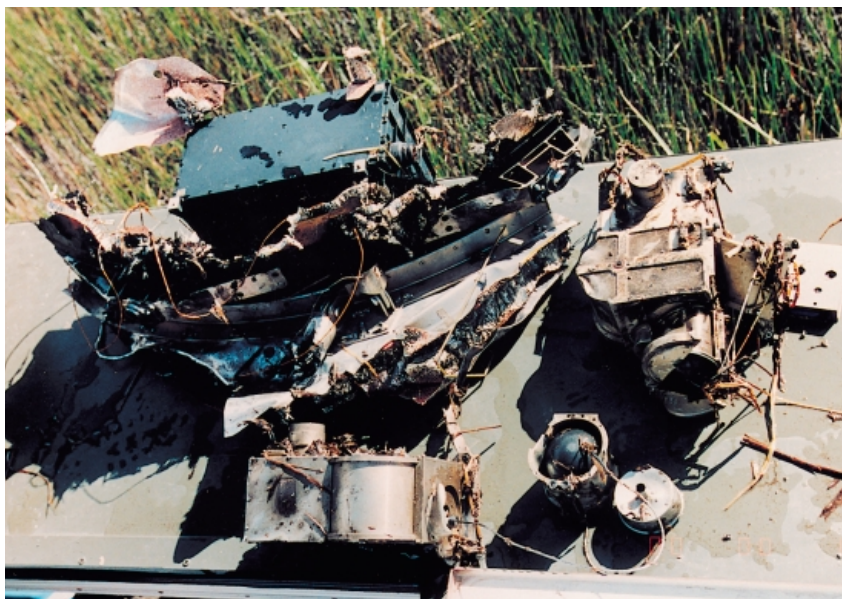
Figure 2. Debris from the Cluster spacecraft being collected after the Ariane-501 launch failure
