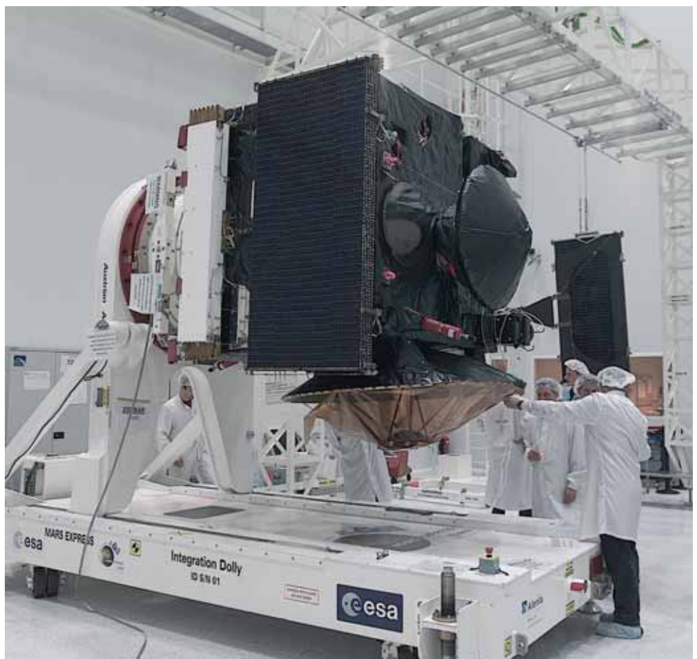
The Mars Express spacecraft with its solar arrays and thermal blanket installed; Beagle is visible on the right-hand side of the craft
