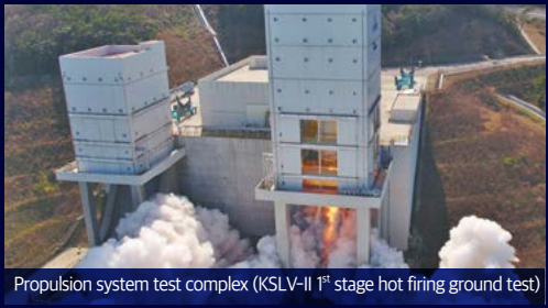
Propulsion system test complex (KSLV-II 1 st stage hot firing ground test)
