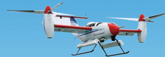
Tilt-Rotor UAV (TR-60) Length : 3 m Max. speed : 250 km/h Max. take-off weight : 210 kg Endurance : 5 hours
