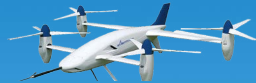
Quad Tilt Prop-UAV (QTP-UAV) Length : 2 m Max. speed : 160 km/h Total Weight : 48 kg Payload : 3 kg Endurance : 30 minutes (battery), 2 hours (hybrid)
