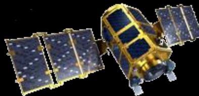
KOMPSAT-2 Design lifetime : 3 years 2006.7.28 ~ 1.0 m EO Payload LTAN : 10:50
