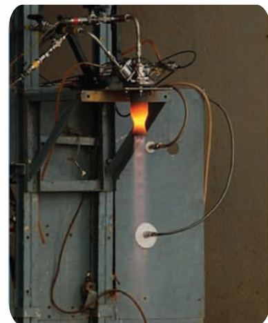
Liquid Engine undergoing sea level hot test at TERLS
